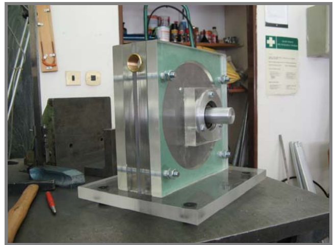
Pict. No. 2 Design of Tesla turbine.
